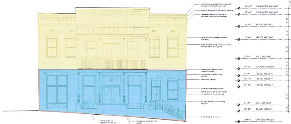
1 WEST EXTERIOR ELEVATION 3/16"=1'-0"
