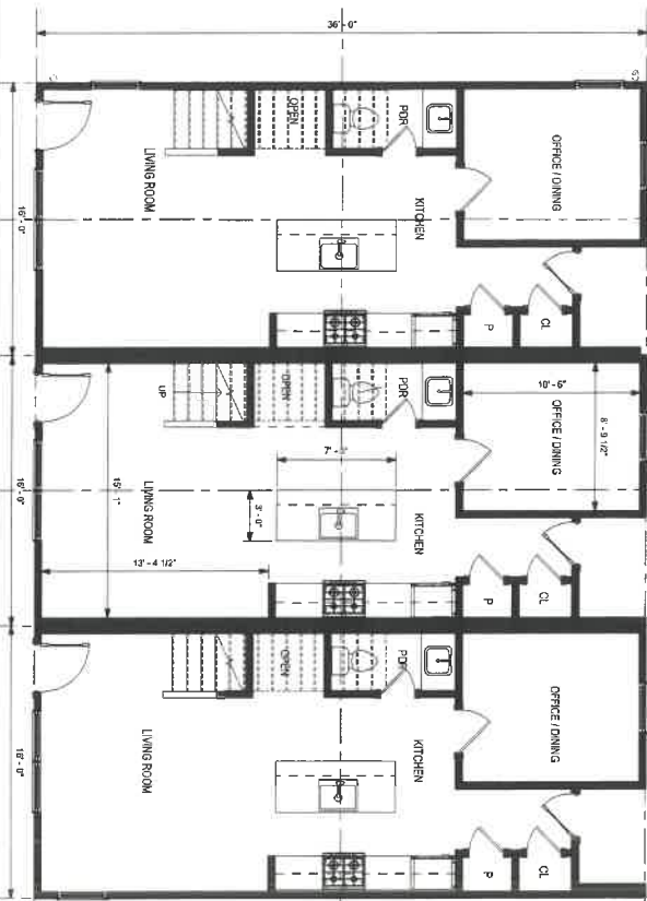
1 FIRST FLOOR PLAN 1/4" = 1'-0"
