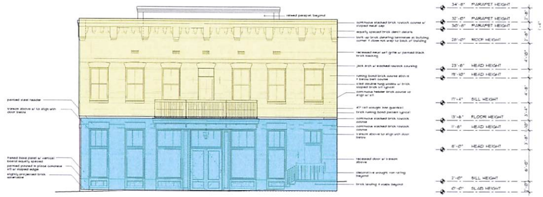
1 EAST EXTERIOR ELEVATION 3/16" = 1'-0"
