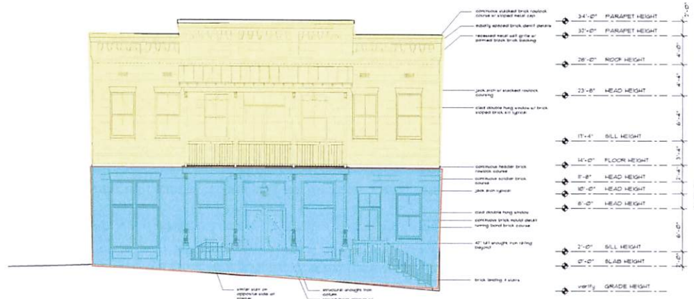
1 WEST EXTERIOR ELEVATION 3/16" = 1'-0"
