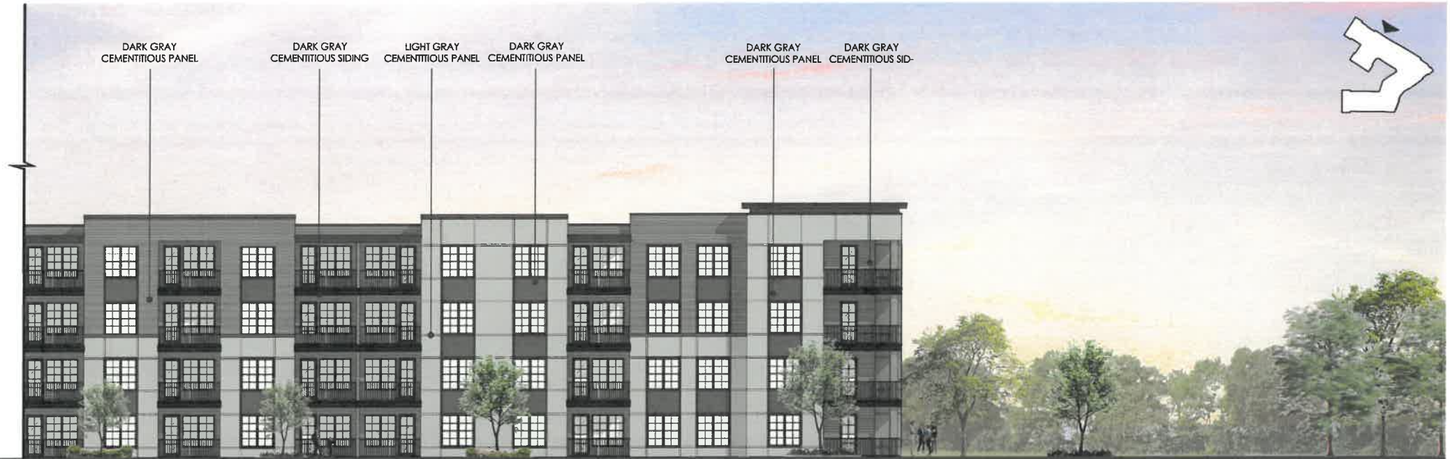
BLDG 1000 - NORTH ELEVATION SCALE: 1" = 3/32"
