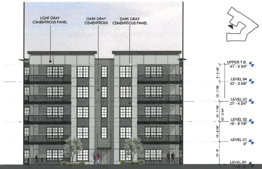
BLDG 1000 - NORTH-WEST ELEVATION SCALE: 1" = 3/32"
