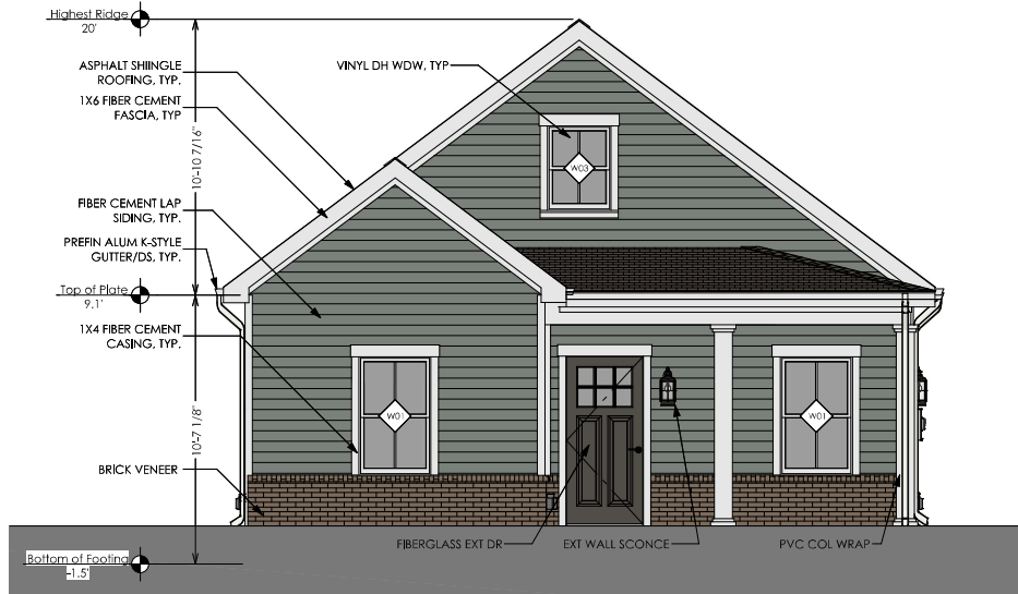
1 FRONT ELEVATION SCALE: 3/16 in = 1 ft
