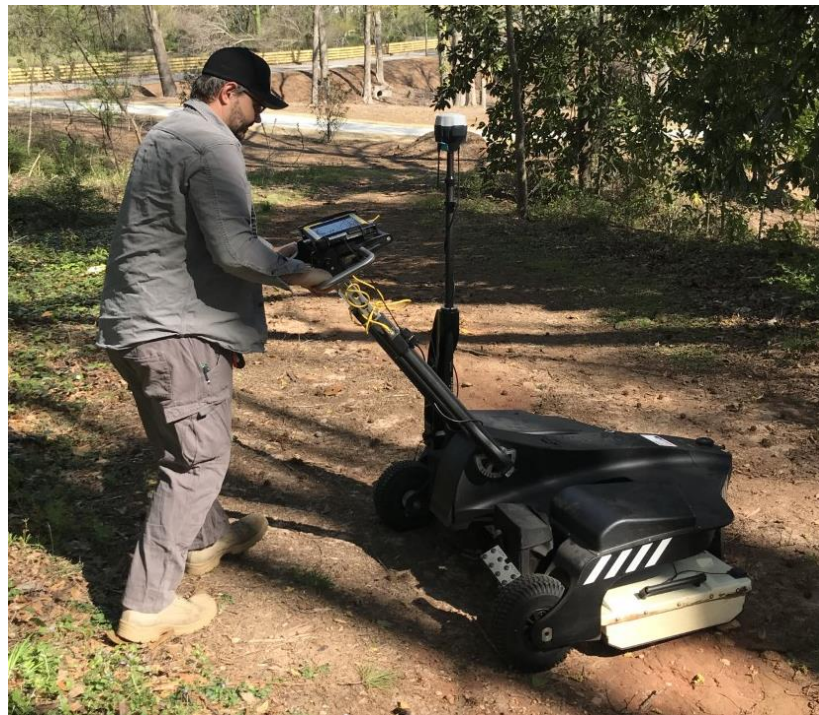
Figure 2: The GPR and GPS Rover deployed on site.
