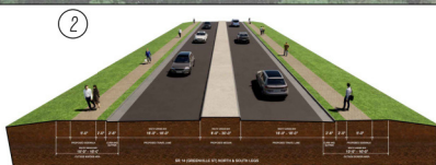
TYPICAL SECTION - GREENVILLE ST.
