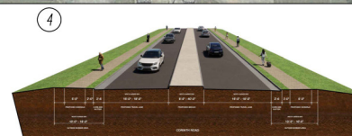
TYPICAL SECTION - CORINTH RD
