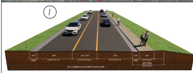
TYPICAL SECTION - GREENVILLE ST.
