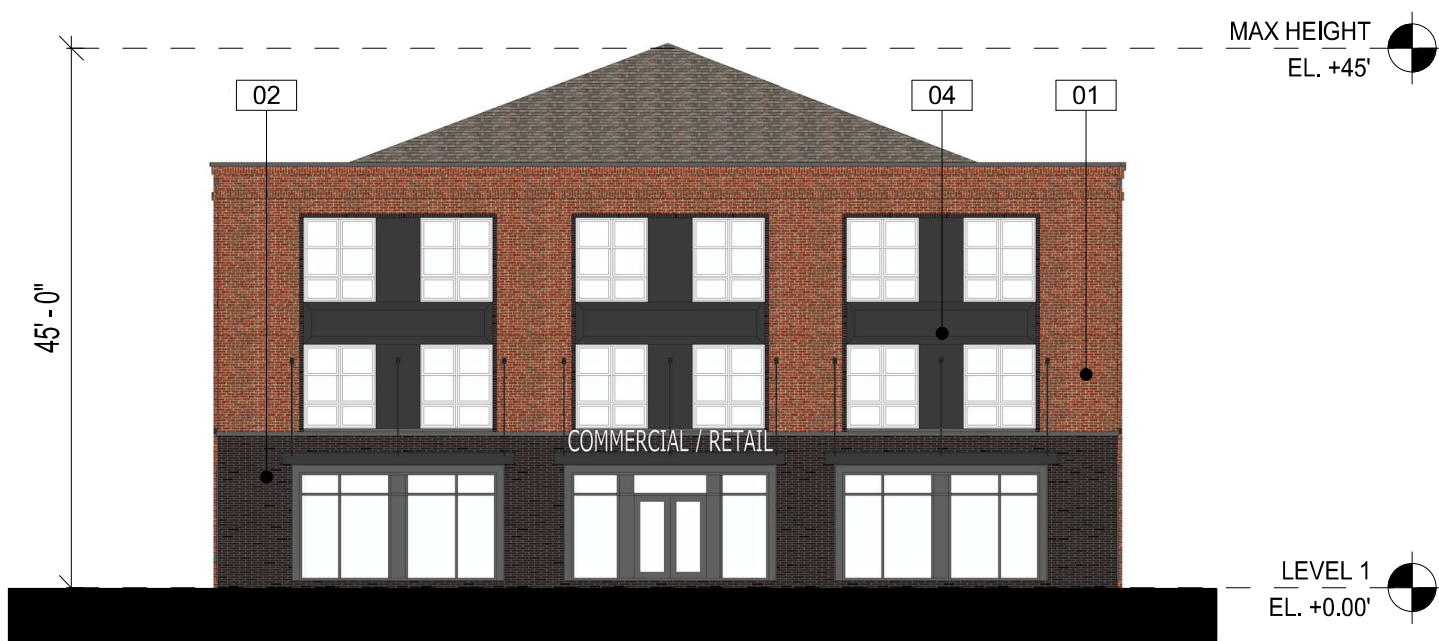
3 B2-3_ Front Elevation A5.2.0 SCALE: 1/16" = 1'-0"
